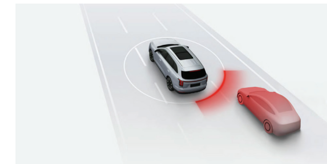
Blind Spot Detection (BSD) Monitors vehicle side blind spots continuously and alerts the driver when other vehicles enter.
