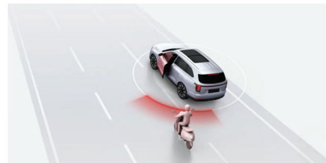
Door Open Warning (DOW) Monitors approaching vehicles or pedestrians from the rear sides and alerts occupants before opening the door.
